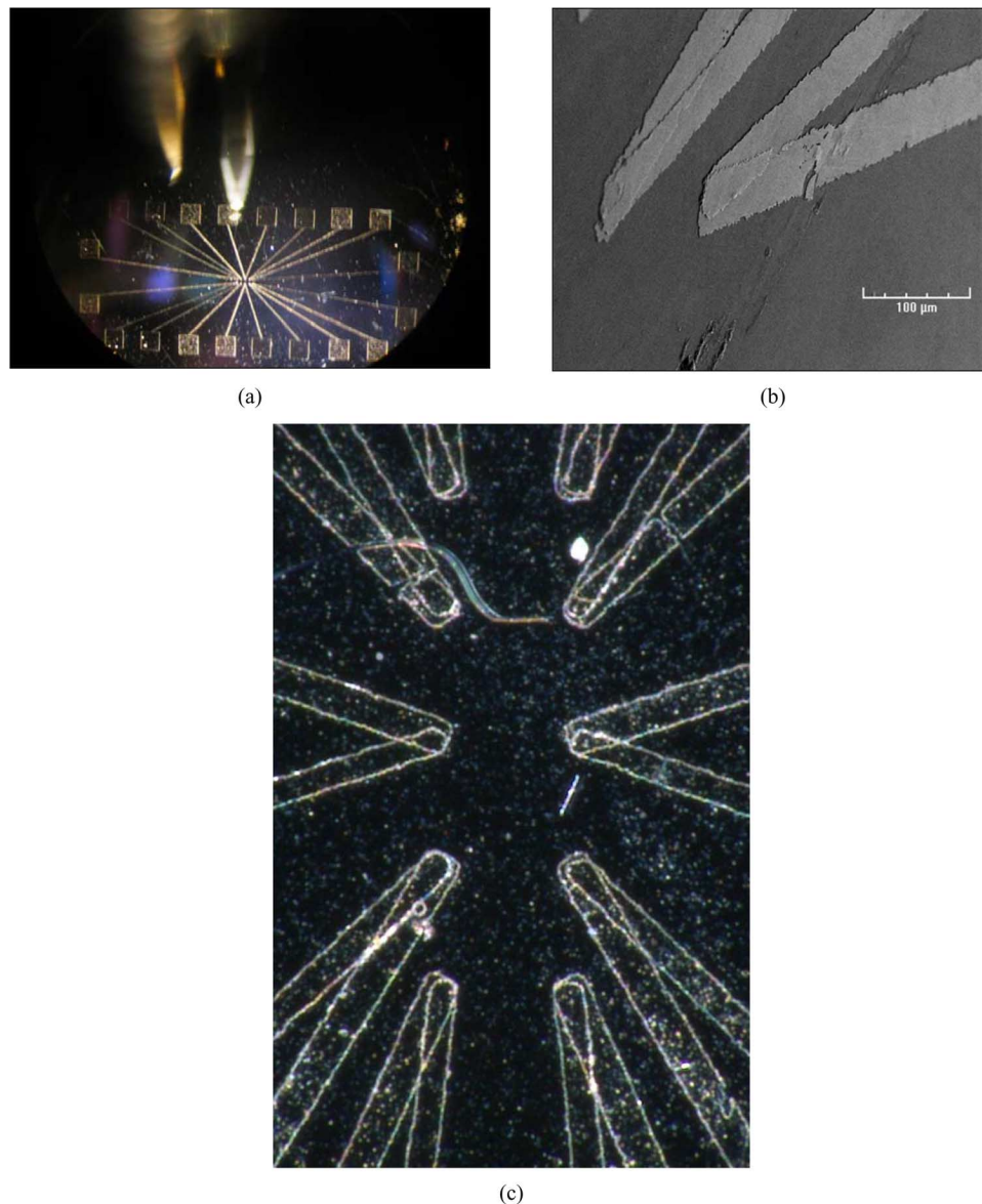
Fig. 2. (a) Optical microscopy image of TFT junction (observed in the wire bonder instrument). (b) SEM Image of TFT junction showing two TFT junctions formed by overlapping the two conductor layers (chromel and alumel). (c) Image taken using a microscope, showing all the ten junctions (alumel–chromel junctions) of the array.
