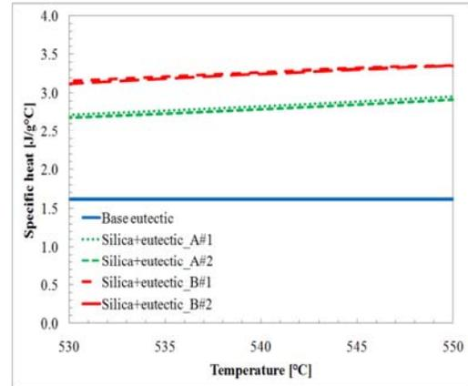
Figure 3. Variation of specific heat capacity with temperature for pure eutectic sample and nanofluid samples (liquid phase data).
