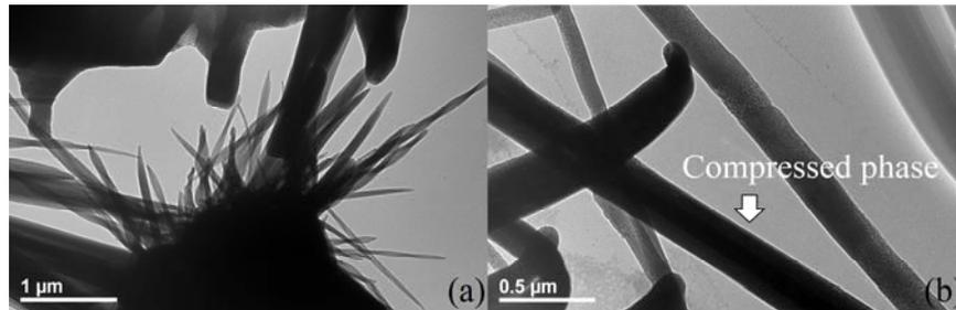
Figure 5. TEM images of the Type-B samples. Needle shaped structures (compressed phase) were induced within the solvent material by the nanoparticles, where the diameter of the needle shaped structures is  $\sim 200 - 400$  nm.
