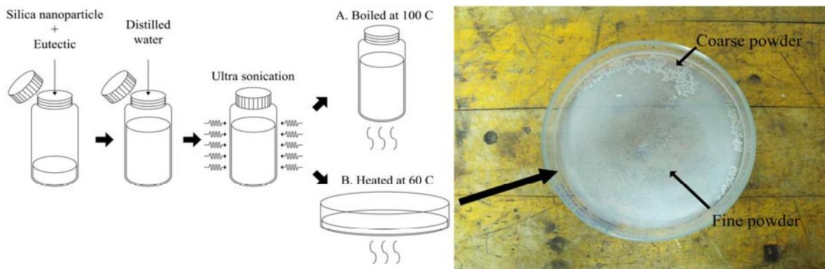
Figure 1. (a) Schematic for the two protocols explored in this study for synthesis of nanomaterials.
