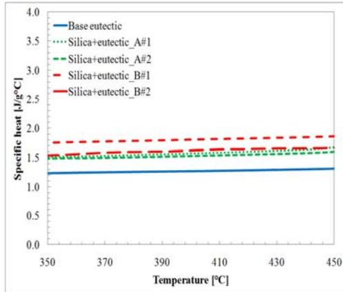
Figure 2. Variation of specific heat capacity with temperature for pure eutectic sample and nanocomposite samples (solid phase data).
