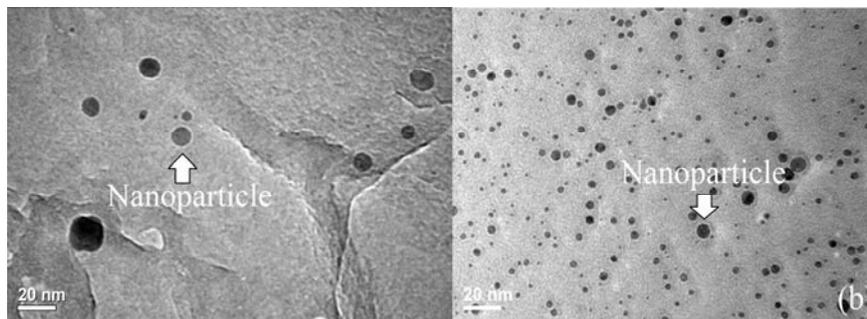
Figure 6. (a) TEM images of silica nanoparticles in the Type-A samples. (b) TEM images of the silica nanoparticles in the Type-B samples. Both images were obtained after multiple freeze/ thaw cycles from the thermo-cycling experiments performed in the DSC.
