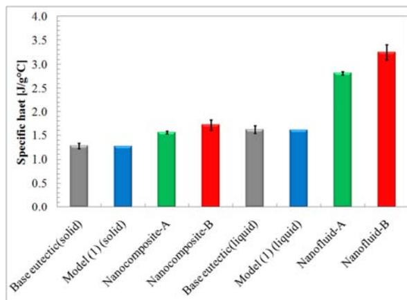
Figure 4. Comparison of experimental data with predictions from Model 1.
